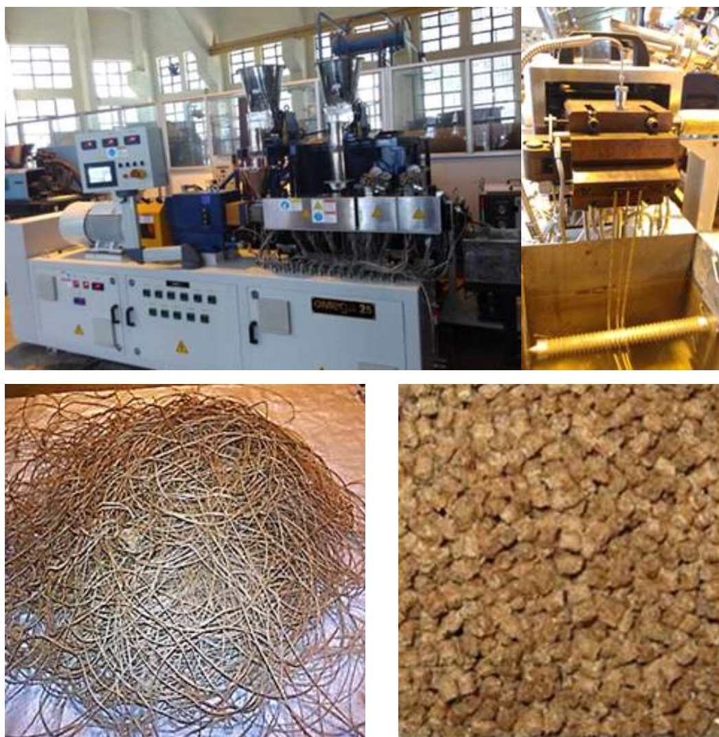
Fig.3: Lantana-polypropylene composite strands (left) and pallets (right)
