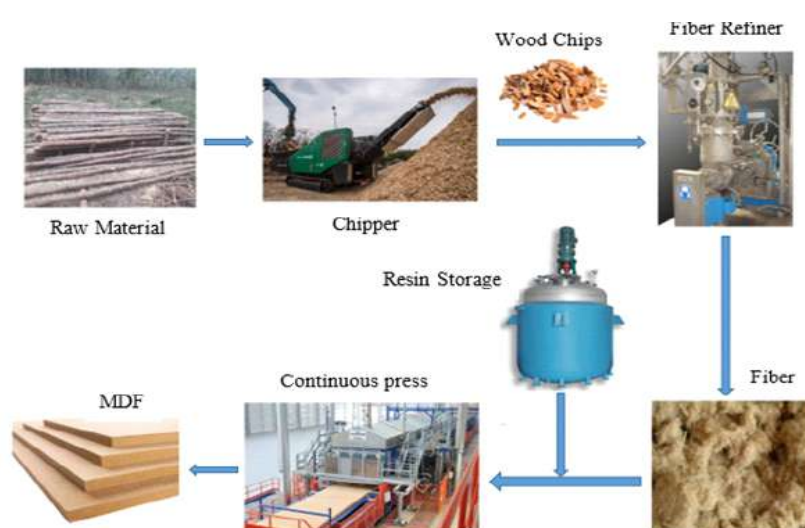
Fig 3. Pictorial flow chart of MDF manufacturing
